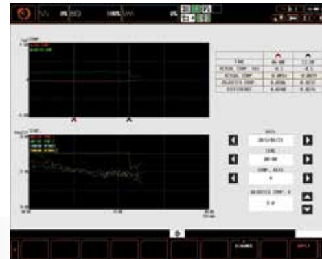
Temperature and compensation is displayed on screen. Operator can adjust compensation by looking at the data.
