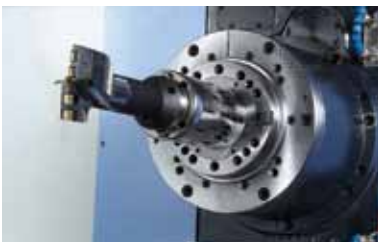
High-torque spindle head for heavy duty cutting
