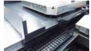
Chip pan Slope-type pan for smooth coolant drain and chip disposal.
