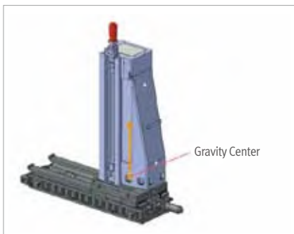
Design focused on low center of gravity of column to minimize vibration during column travel.
