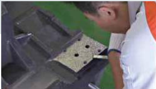
100% Hand-Scraping for Geometry Accuracy and Rigidity
